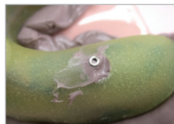
Area of exposed guide pin head
