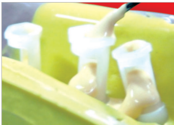
Fine injection of mixed plaster into the analog
