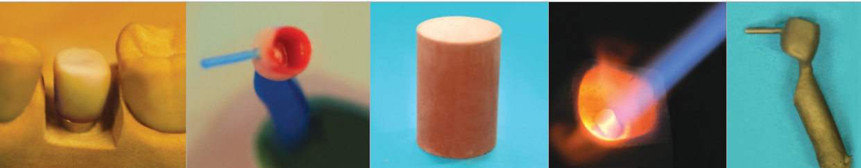
Copping wax-up Spruing Investment Casting Casting body
