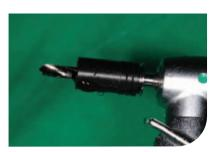
• Ø 2.8 → Ø 3.1 CAS-Drill (800rpm) A 5mm Stopper is used for the final drilling and lifting of the membrane.
